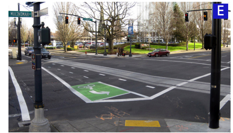
Example of a two-stage turn queue box.
